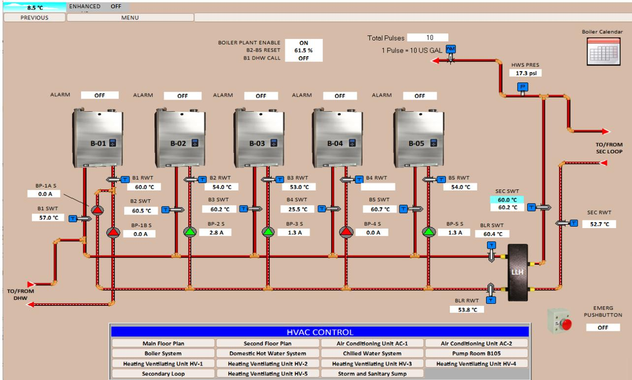
Figure 1: Boiler plant in the DDC
