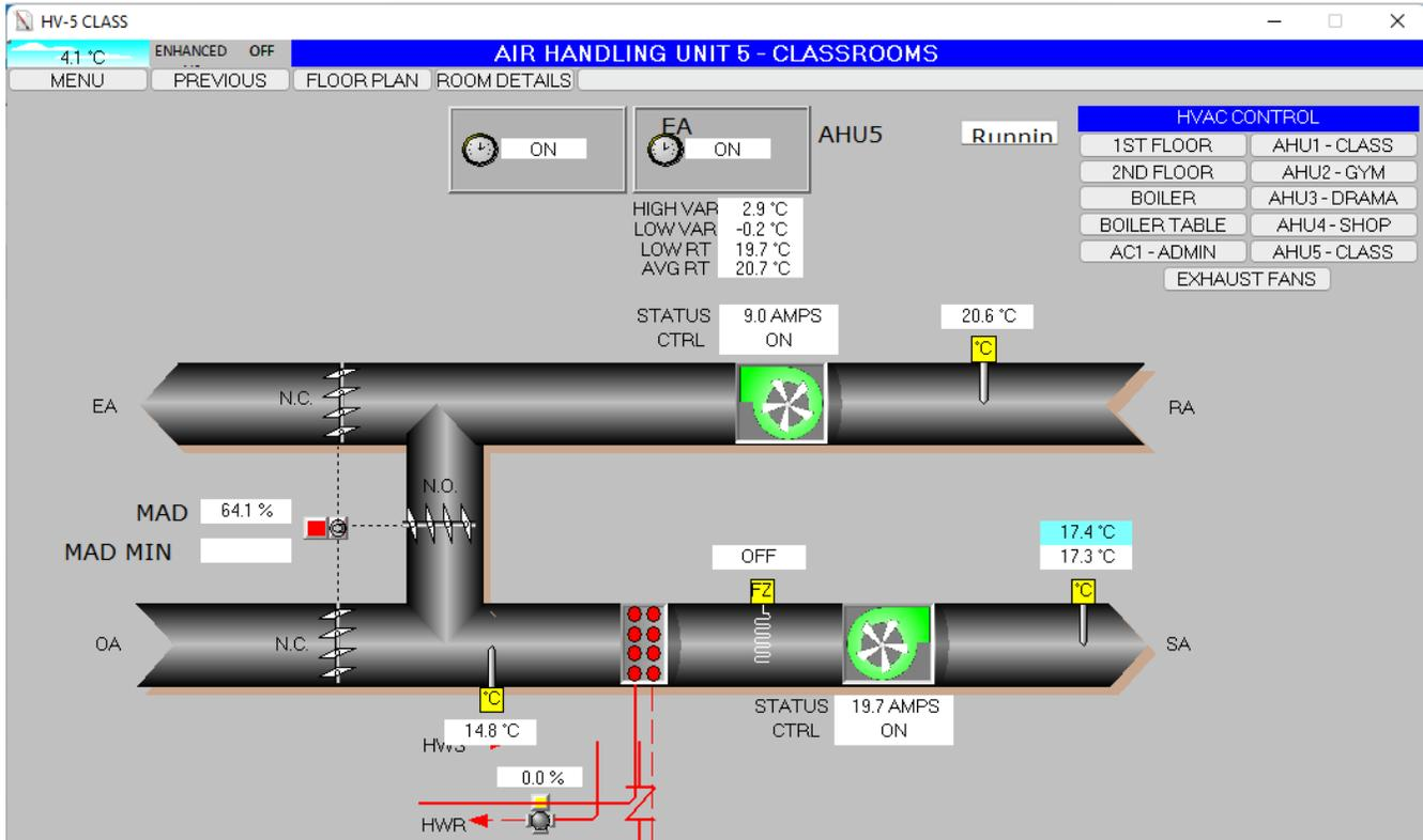
Figure 3: AHU-5 heating despite the control valve closed.
