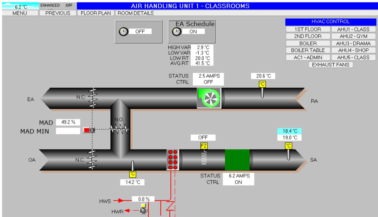
**Figure 5: AHU-1 runs with open mixed air dampers even when the main schedule is OFF**
