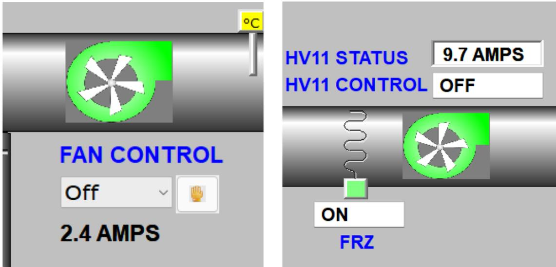
Figure 9: HV10 (left) and HV11 (right) supply fans
