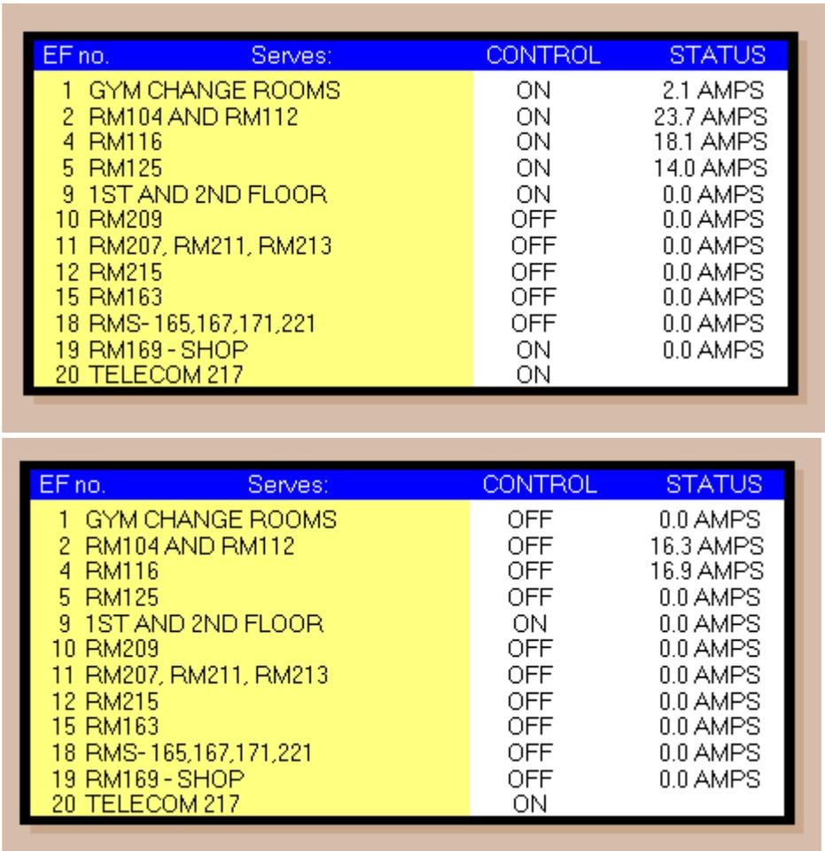
Figure 18: Exhaust fans at different times
